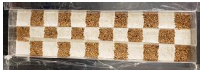
Figure 4.1. Image of the dispersal landscape used to separate high and low dispersers and measure dispersal variables. The arena consisted of three adjacent 60 x 5 x 5 cm rectangular prisms that connected to each other and allowed a beetle to move a maximum distance of 180 cm. The white squares are habitable patches of flour whereas the brown squares are less habitable areas of whole wheat berries.
